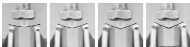
Figure 16 Illustration of failure progression of lubricant oil soaked specimen.
