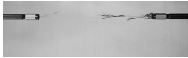
Figure 14 Typical tensile failure modes of oil soaked + thermal cycled composite rods.
